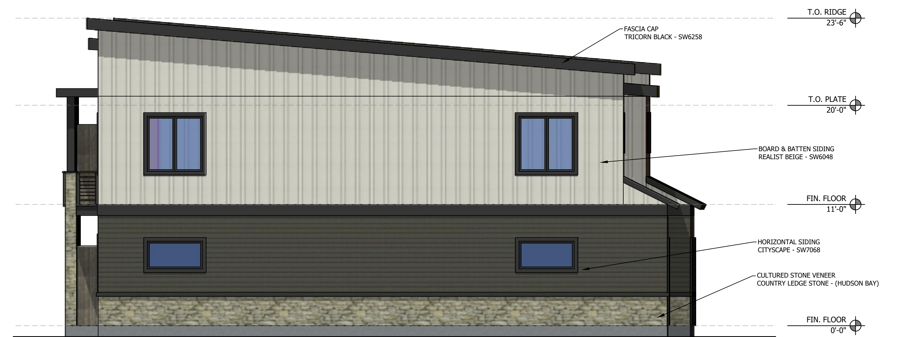
EXTERIOR ELEVATION - SIDE
